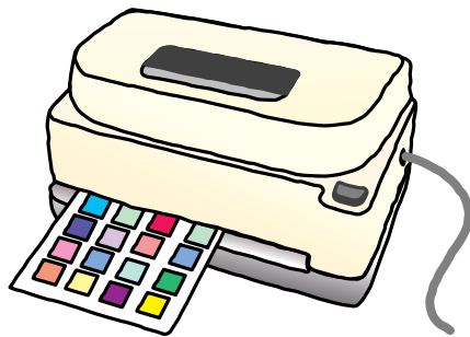
The X-Rite DTP-41 auto scanning spectrophotometer can shorten the time needed to read the hundreds of patches produced when profiling a printing machine.
