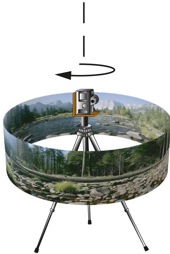
With the tripod and its rotating index head, the camera is panned through a series of frames to take the entire panorama. In this illustration the arrow indicates a clockwise rotation, but the direction is unimportant.
